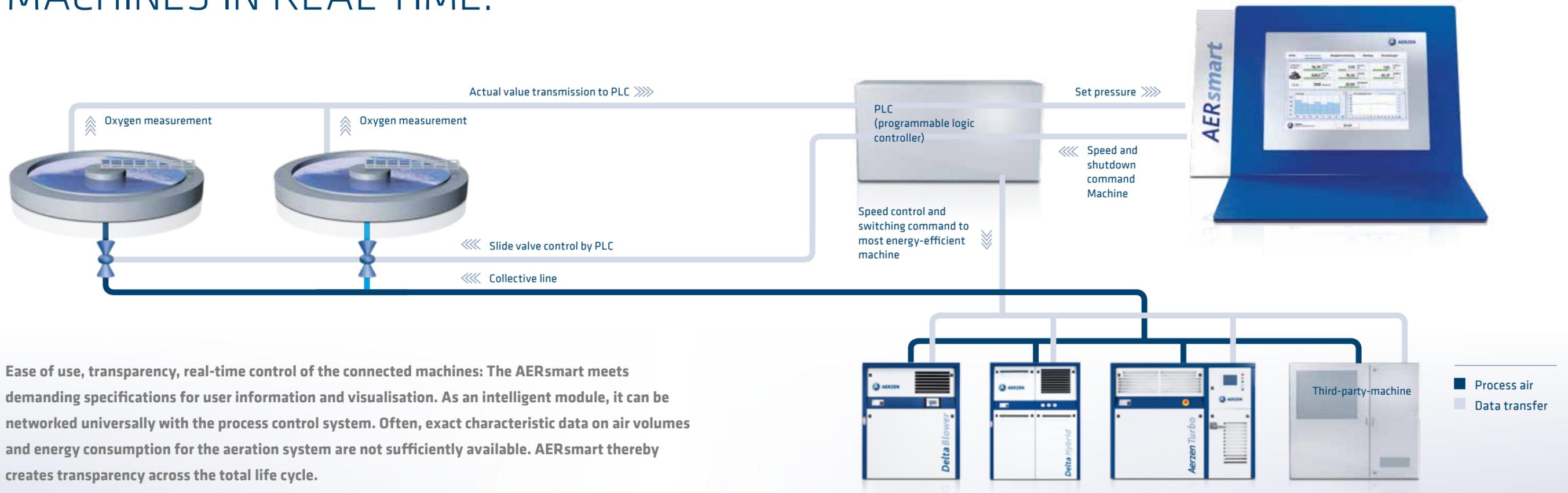
Ease of use, transparency, real-time control of the connected machines: The AERsmart meets demanding specifications for user information and visualisation. As an intelligent module, it can be networked universally with the process control system. Often, exact characteristic data on air volumes and energy consumption for the aeration system are not sufficiently available. AERsmart thereby creates transparency across the total life cycle.
