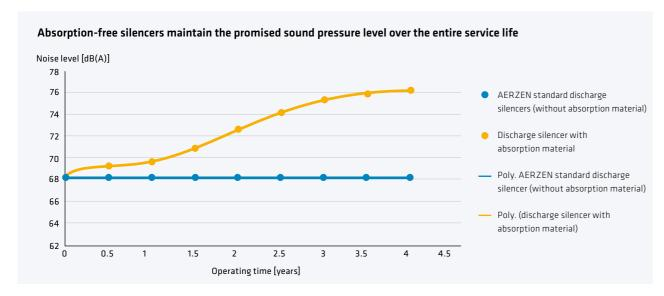
Noise development due to wear of the absorbent in the discharge silencer Pipe sound level at constant volume flow  $30 \text{ m}^3/\text{min}$  at 600 mbar (q)
