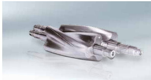
3+3 blower profile with twisted rotors and patented pre-compression by pulse-charging as well as reduced losses caused by trapped air in the rotor valleys
