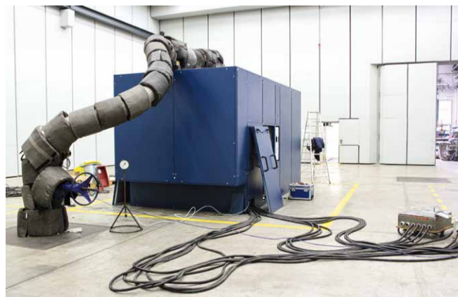
The Delta Screw package VML 250 during the function test in the AERZEN Acoustics Hall
