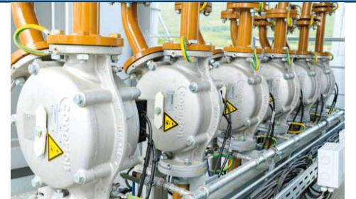
The pulverised lignite is blown through burner lances into the kiln by AERZEN Delta Blowers.
