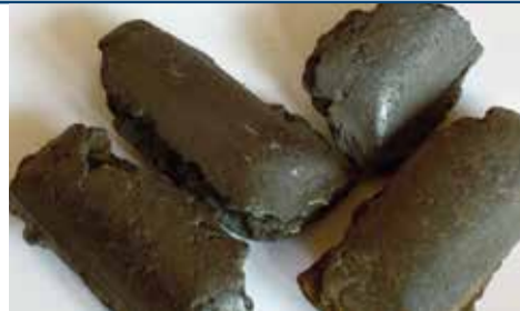
In direct reduction processes, briquettes of sponge iron are being made.
