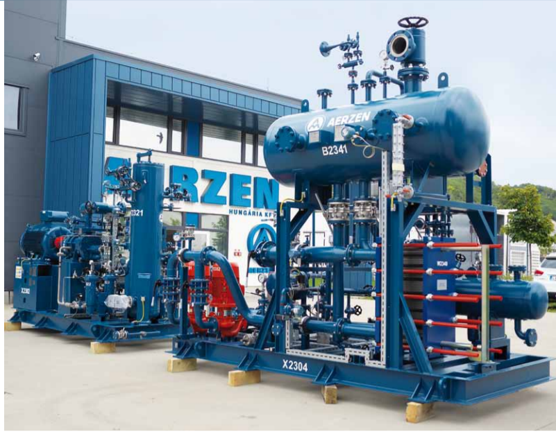
The PGD competence centre in Hungary is seeing growing demand for AERZEN products in Western Europe. This is a chlorine liquefaction plant for a system manufacturer in Germany.
