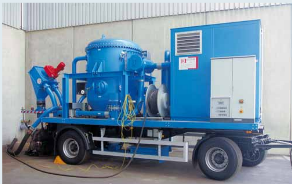
Vacuum cleaning system manufactured by Messrs. IB process technology. A positive displacement blower of Aerzener Maschinenfabrik, located in a sound-insulating housing at the front of the vehicle, produces the necessary negative pressure.
