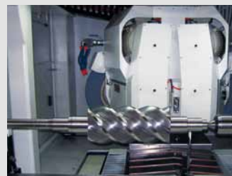
The new Danobat machine grinds compressor rotors to micrometre accuracy.
