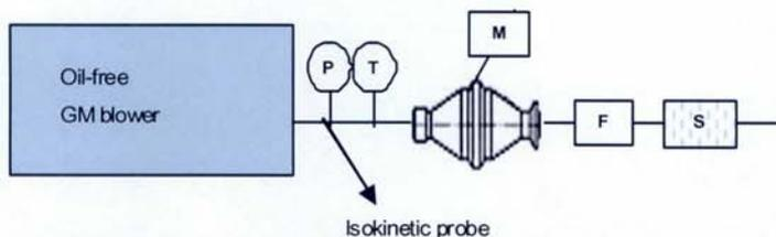
Principle diagram for measurement of oil vapour and organic solvent content as per ISO 8573 Part 5
