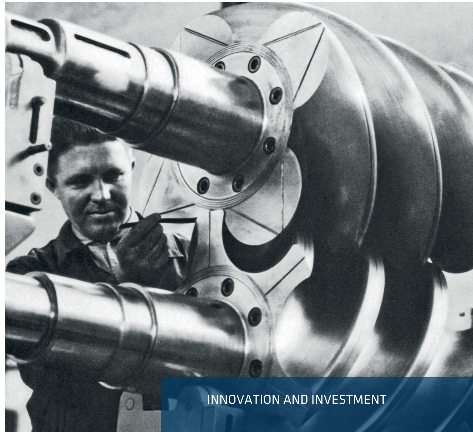
Aerzener Maschinenfabrik also benefits from the sustained growth in West Germany's economy: here a worker inspects screw compressor rotors in the test fixture.
