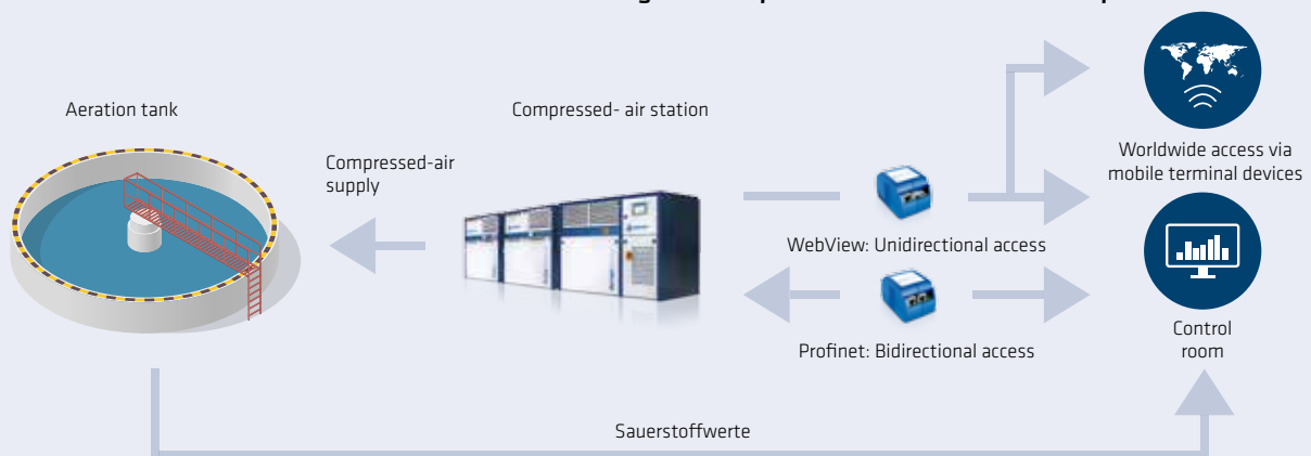
Function method of AERZEN WebView and Profinet using the example of a wastewater treatment plant.
