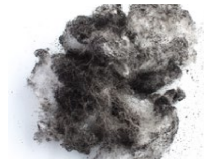
Figure 1: Deposits in bulk material, which collect in silencers with absorption material
